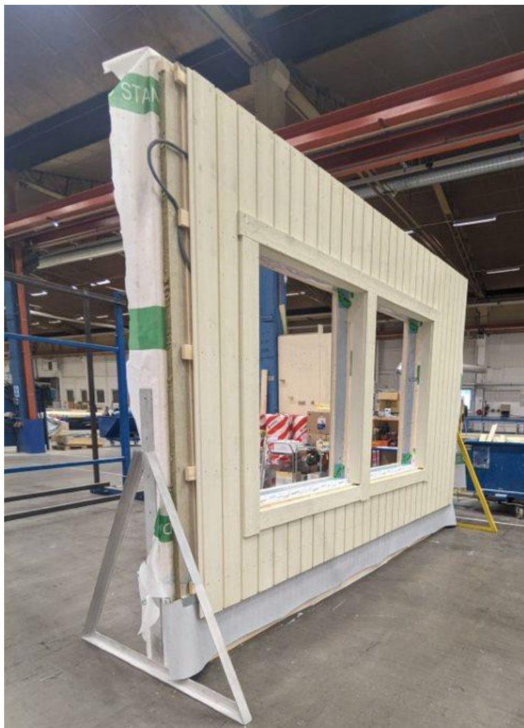
Figure 7 External wall for a module, ready for assembly. Note the thick insulation and double glazing on the windows.
