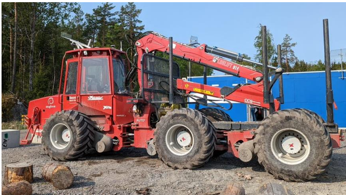
Figure 5 The remotely operable forwarder, put together by Skogforsk .
