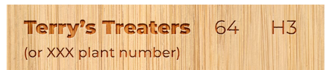
Preservative treated timber (64 is the preservative and H3 is the Hazard Level). Identification may be ink brand or end tag.
