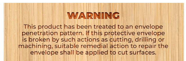
Label where required on envelope treated timber such as LVL, Plywood, Glulam and Reconstituted Wood products. This does not apply to H2F envelope treated framing.
