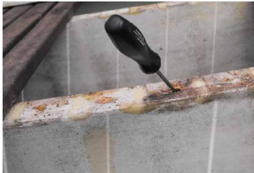
(F17 joists failed in 3.5 years) Victorian Ash – Low durability irrespective of strength
